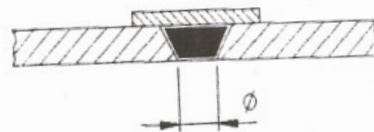
Fig. 11. A set up for filling a hole before welding
