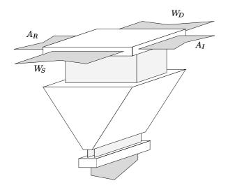
Figure 2: The multiplier for  $Z_R$  or  $Z_I$ , the complete complex multiplier consists of two of these. Partial inner product generator at the top, adder tree in the middle, and fast carry-lookahead adder at the bottom.
