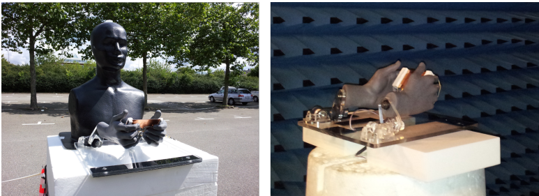
Figure 3.5: Phantom user scenario setups. Propagation measurement in a TH mode with head and torso in an outdoor environment [50] (left). Radiation pattern measurement in a TH mode with phantom hands only [18] (right) ©2013 IEEE.
