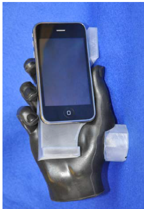
Figure 3.2: IndexSAR CTIA hand phantom [46].
