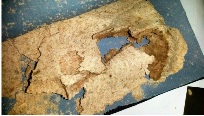
Figure 27 Banana purée dried with a supported SAP pouch in a convective dryer, to simulate an indirect solar dryer without relative humidity control. The drying conditions were 51.4^{\circ}\text{C} \pm 0.1^{\circ}\text{C} , 10.6\%RH \pm 2.3\%RH , and 1.8 \text{ m/s} \pm 0.2 \text{ m/s} .
