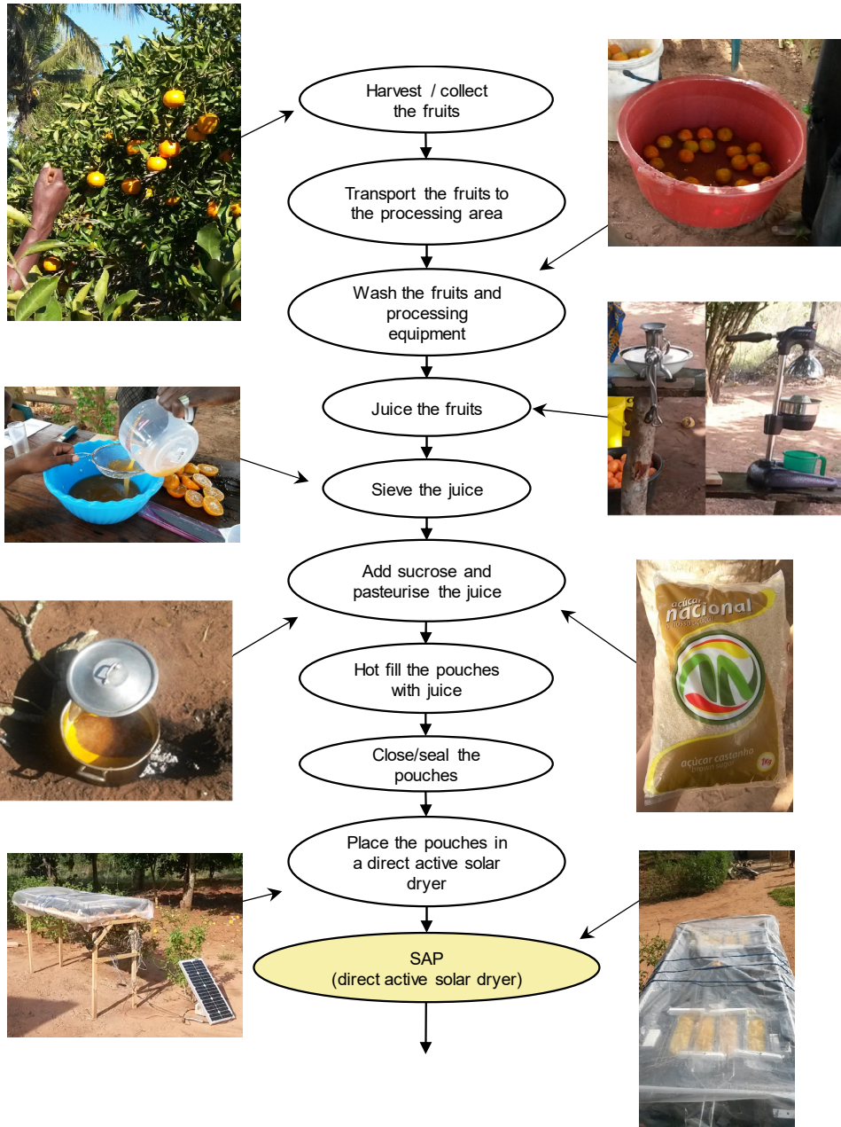
Figure 43 The first part of the recommended SAP process from harvest to Solar Assisted Pervaporation. Larger membrane pouches could be used in the future. All photographs taken by R. Phinney © 2017
