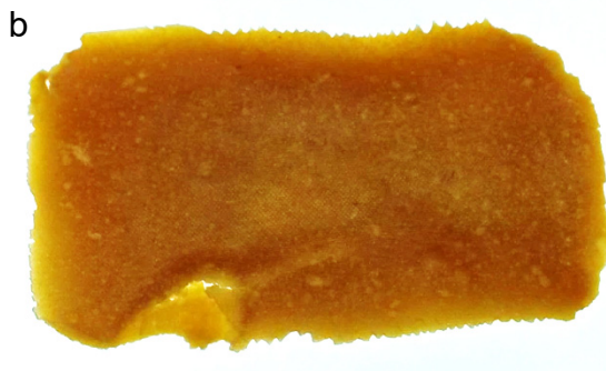
Figure 28 Apple purée dried with a supported SAP pouch in a convective dryer to simulate an indirect solar dryer without relative humidity control. The dried form of the purée is more like a fruit “leather”. a: Sample removed after 10 hours of drying. b: Sample removed after 16.4 hours of drying. The drying conditions were 52.0^{\circ}\text{C} \pm 0.2^{\circ}\text{C} , 10.6\%RH \pm 1.5\%RH , and 1.8 \text{ m/s} \pm 0.2 \text{ m/s} for both a and b.
