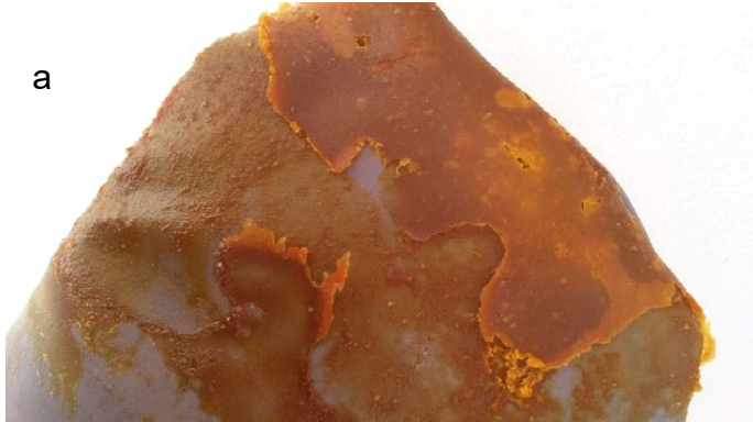
Figure 27 Banana purée dried with a supported SAP pouch in a convective dryer, to simulate an indirect solar dryer without relative humidity control. The drying conditions were 51.4^{\circ}\text{C} \pm 0.1^{\circ}\text{C} , 10.6\%RH \pm 2.3\%RH , and 1.8 \text{ m/s} \pm 0.2 \text{ m/s} .
