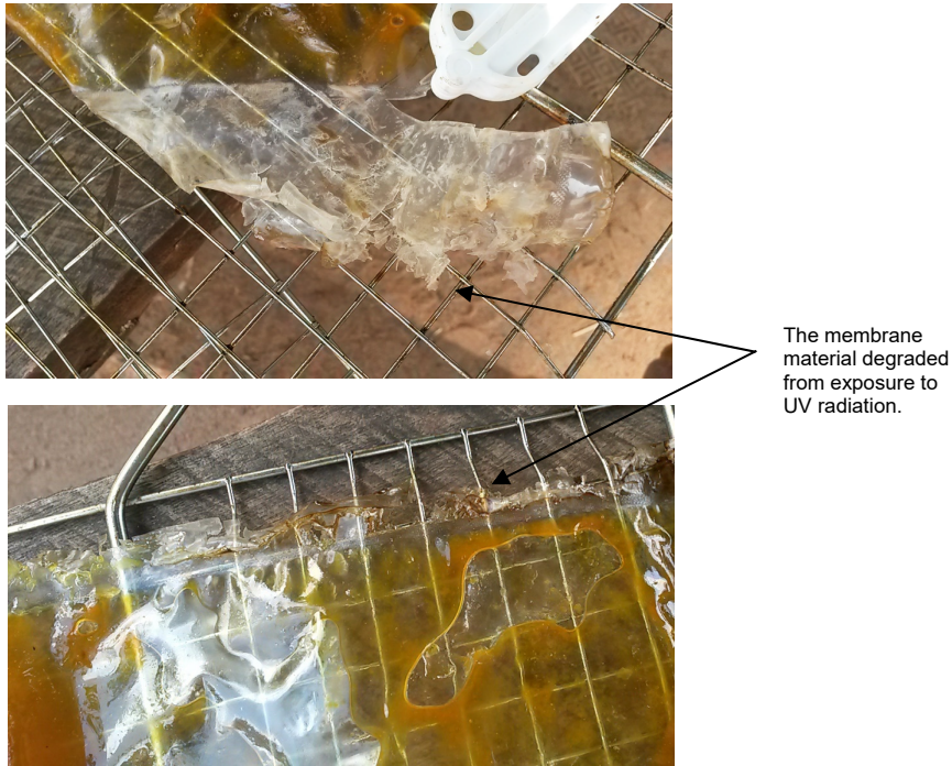
Figure 45 Unsupported membrane pouches that suffered from UV degradation in the direct active and tilted passive solar dryers. © R. Phinney, 2017.
