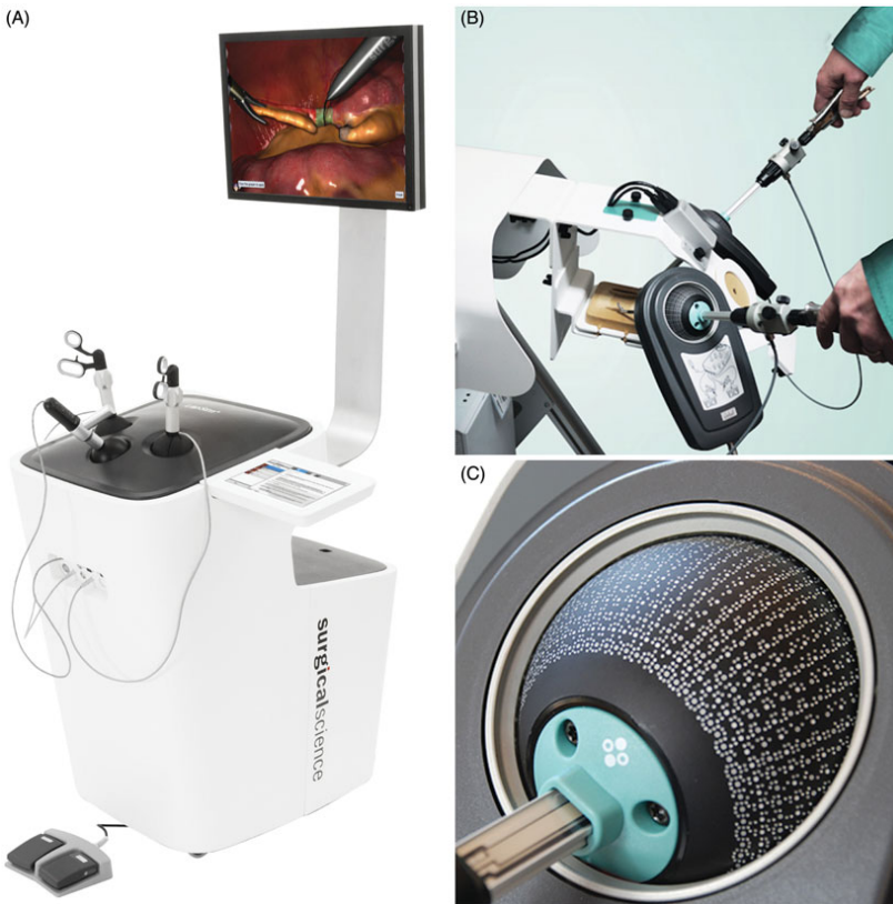
Figure 1. (a) LapSim ® on SimFrame virtual reality simulator with haptic feedback and 3D vision. (b) Simball ® Box video trainer delivering objective metrics on performance using ordinary laparoscopic instruments. (c) Close-up on the Simball ® Box laser-marked pattern in the trocar responsible for recording metrics.
