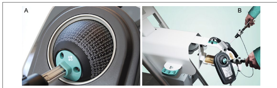
Figure 1. The Simball box. A laser marked pattern on the ball joint's surface forms a dot pattern code with a configuration being unique depending on its position on the ball surface (A). The instrument holder is inserted in the ball joint (A + B) and equipped with a linear potentiometer measuring linear motion of the instrument holder. During box training authentic surgical instruments are inserted and fixed in the instrument holder (B).
