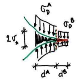
$K_{I} = 2\sqrt{\frac{2}{\pi}} \left[ \sqrt{d^{4} + d^{6}} \mathcal{T}_{p}^{A} - \sqrt{d^{6}} (\mathcal{T}_{p}^{A} - \mathcal{T}_{p}^{B}) \right]$
