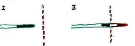
3. Initiation of Crack Growth from Interf.
