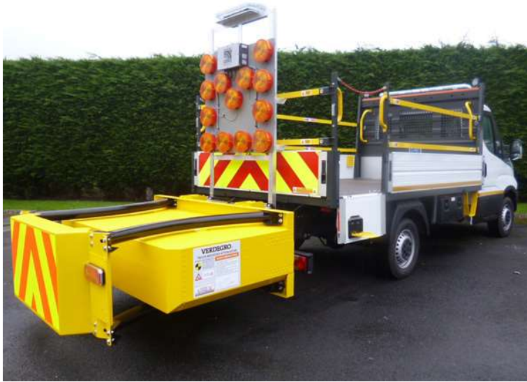
Figure 32: TMA, equipped with crash cushion and various LEDs (beacon bars, work lights, strobes)
