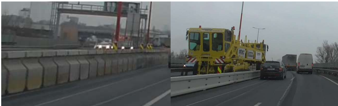
Figure 26: Quick moveable barrier and vehicle for application/moving of barriers
