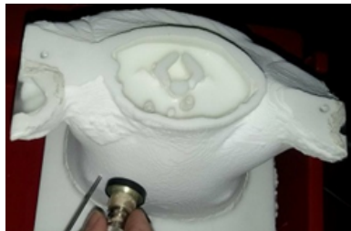
Figure 4.4: Picture of the 3D-printed phantom with the liquid phantom filled into the hollow organs.
