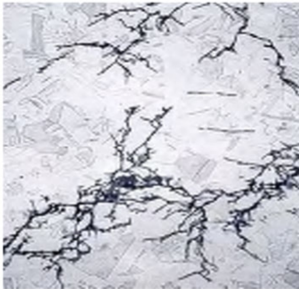
Corrosion in stainless steel caused by Gallionella Bacillus. ASTM.
