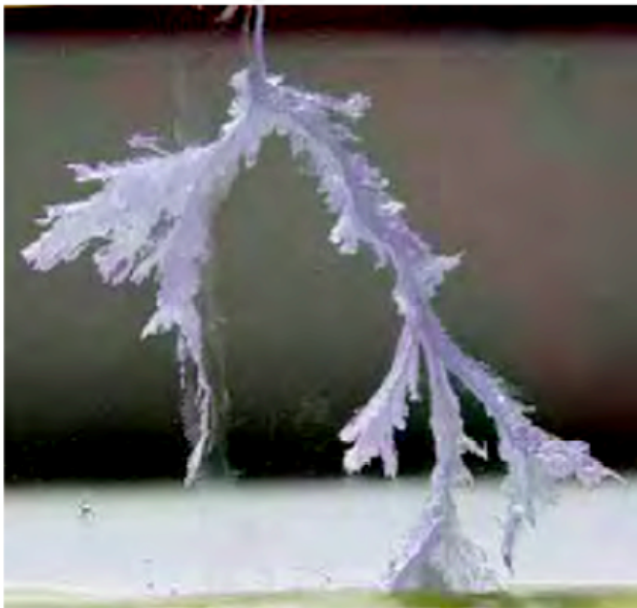
Growing crack in a polycarbonate exposed to acetone (Hejman 2011)
