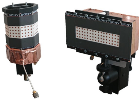
Figure 8: Left: 256 element receiver array. Right: 128 element transmit array.
