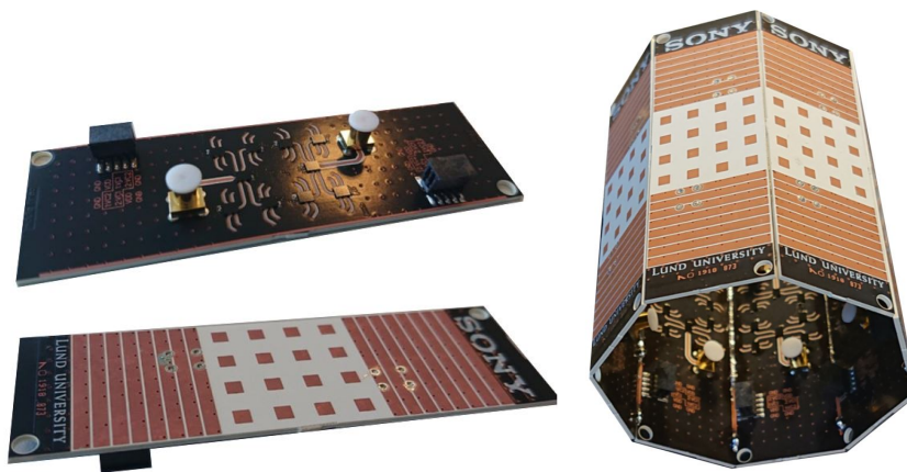
Figure 3.16: To the left, antenna panels before assembly. To the right, antenna panels assembled into the octagonal shape.
