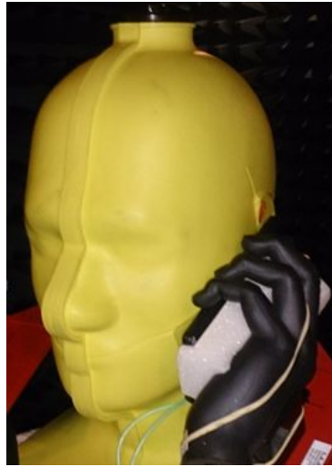
Figure 3: Phantom head with hand left.
