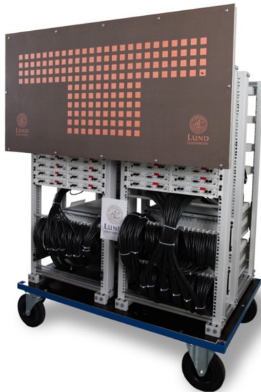
Figure 3.10: The Lund University Massive MIMO testbed.
