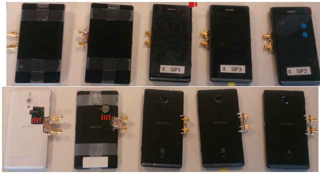
Figure 3.3: Five prototypes based on Sony Xperia-ZL and -SP chassis. The top picture shows the fronts and the bottom picture the rear of the same prototypes. The two prototypes to the left are the based on the Xperia ZL and have four antennas integrated. The three prototypes to the right are based on Xperia SP and have two antennas each.
