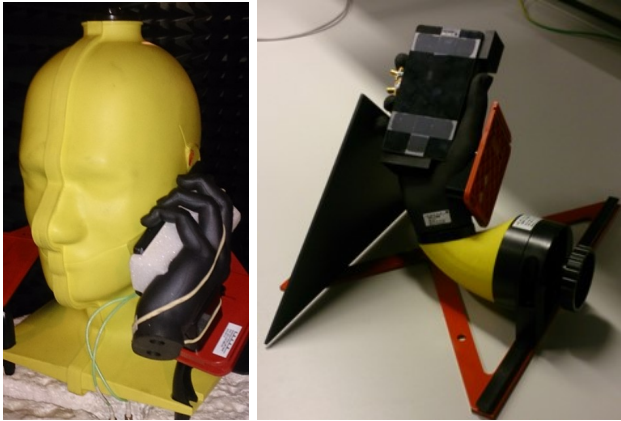
Figure 3.2: Phantom head with hand left (BHHL) and phantom hand left (LH) fixtures.
