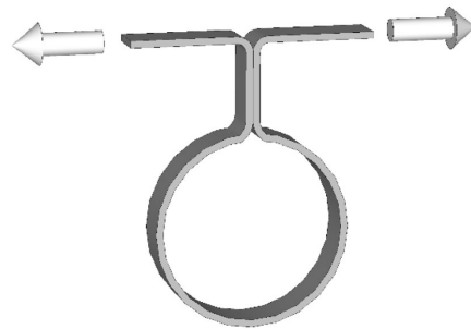
Fig. 2 Rubber-adhesive adhesion tensile test. Bonded area was 50 \times 50 \text{ mm}^2
