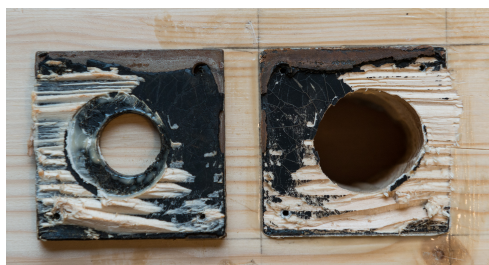
Figure 5: Illustration of different bond line failure modes of the SPDJ. Failure includes shallow wood shear failure (50%), failure in the adhesive layer including the interlayers (30%) and vulcanization failure (20%). Rubber failure of the tensile type seen here occurred during specimen disassembly, after the tests. The steel plate was intentionally mounted eccentric over the over-sized timber hole in order to facilitate a large enough displacement at failure to register the event in the failure detection system. This specific specimen was in group Par-60, see Table 2.
