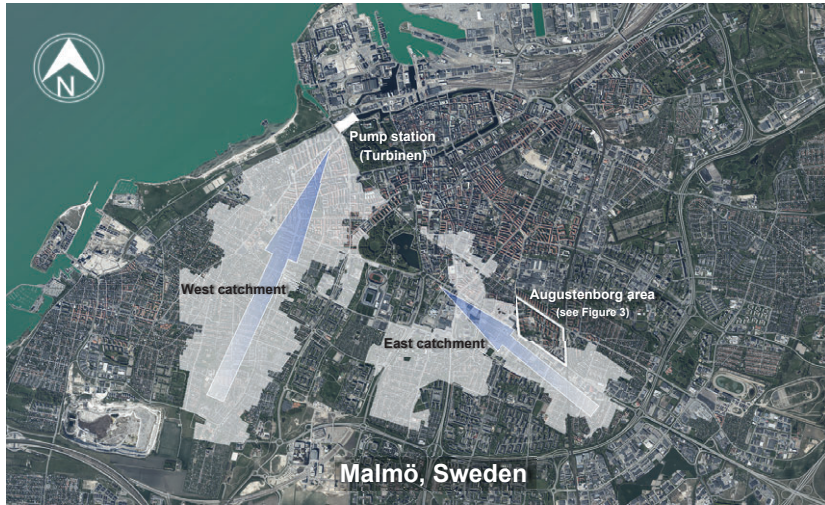
Fig. 2. The catchment area, encompassing 954.35 ha, connected to the combined sewer network in Malmö, Sweden, drained through the Turbinen pump station. Background picture: GSD-Orthophoto, courtesy of The Swedish Mapping, Cadastral and Land Registration Authority, ©Lantmäteriet.
