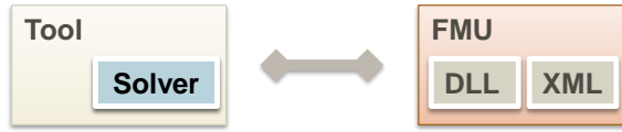
Figure 2.3: A model exchange FMU and the connection to a tool for simulation. Note that the solver is outside of the FMU.
