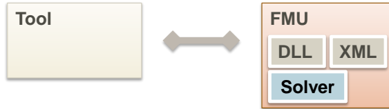
Figure 2.4: A co-simulation FMU and the connection to a tool for simulation. Note that the solver is inside the FMU.
