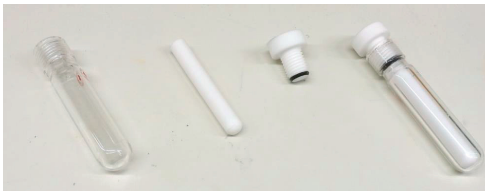
Figure 20. From left to right: an empty glass pressure tube, a Teflon inner tube, a front seal and an assembled holder for the alkaline stability study.
