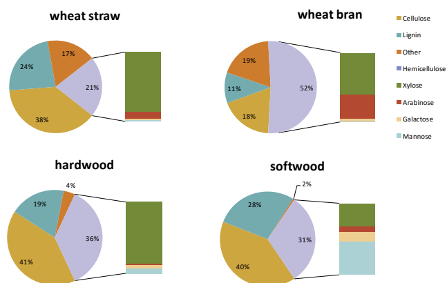
Figure 2. Cell-wall components (cellulose, hemicellulose and lignin) and hemicellulose composition for a variety of biomass, i.e. wheat straw (Lynd et al. 1999, Wiselogel et al. 1996), wheat bran (Immerzeel et al. 2014, Merali et al. 2015), hardwood (birch; Betula pendula ) (Garrote et al. 1999, Lehto and Alen 2013), softwood (spruce; Picea abies ) (Fengel et al. 1989, Willfor et al. 2005).
