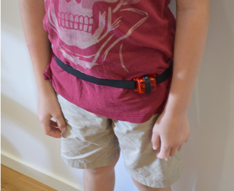
Figure 4. A child wearing the MTI accelerometer model 7164 that was used in the POP-study
