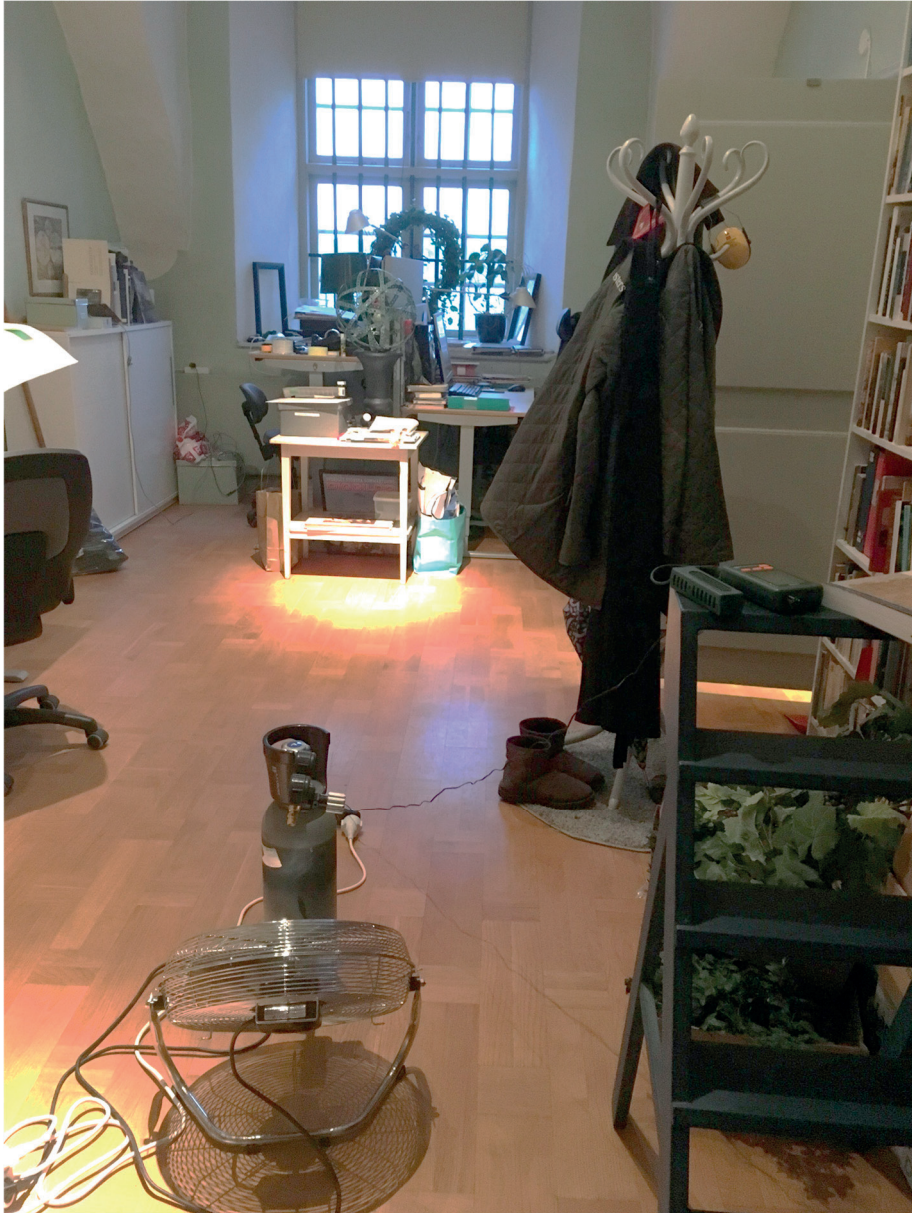
Figure A4.1: Tracer-gas-decay measurement for ACR.
