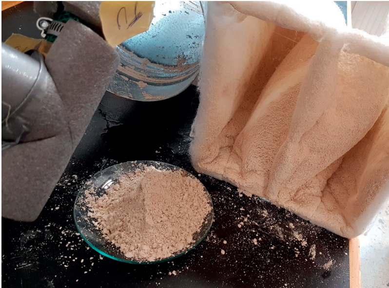
Figure A3.3: Collection of contaminants not stuck on heat exchanger in laboratory tests.
