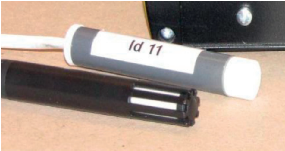
Figure A1.7: Taken from Melorose et al. (2015). Hygrothermal monitoring equipment from SensiLog. The sensor case marked Id 11 is for placement inside porous building materials, while the other sensor case is for monitoring air (such as in cavities, indoor air, etc.). Both use sensors of type SHT75 from SENSIRION.
