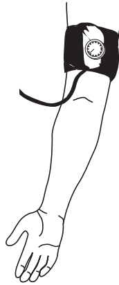
Figure 1.18: Illustration of a cuff for brachial pressure measurement.
