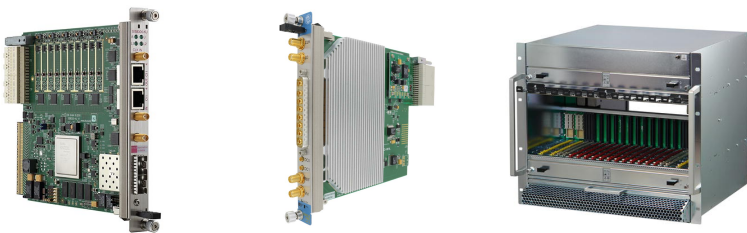
Figure 5.4 Components of an LLRF system based on the MicroTCA standard. Left: Digitizer SIS8300-KU, containing ADCs and an FPGA (Struck). Middle: Signal conditioning board DWC8VM1, containing analog down- and upconversion (Struck). Right: 12-slot MicroTCA4 crate (Schroff). Photo Credit: Struck Innovative Systeme GmbH, and nVent Schroff.
