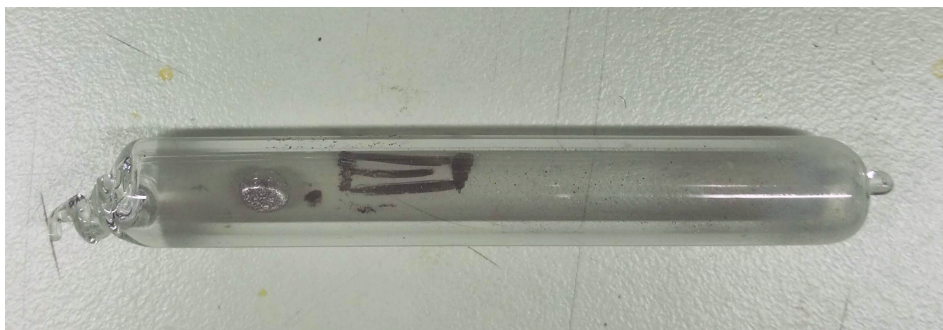
Figure 16: Example of a quartz ampule with a synthesised ingot inside.
