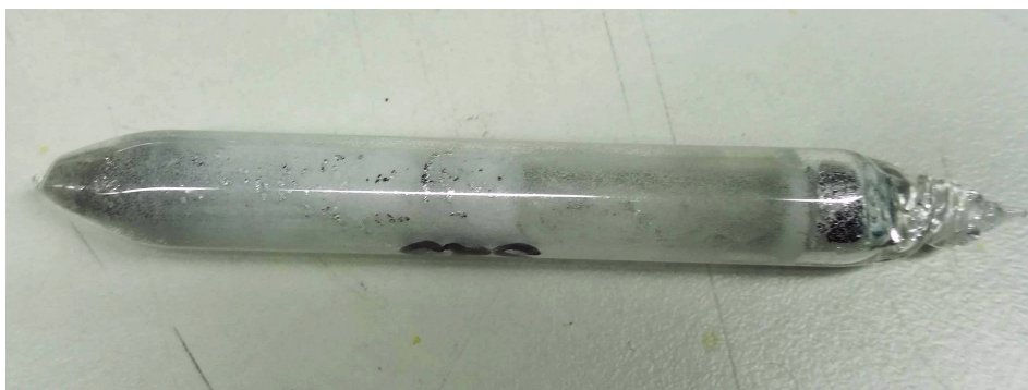
Figure 17: Example of a quartz ampule containing (from left to right) crystalline sample, quartz wool, quartz shards and excess tin.
