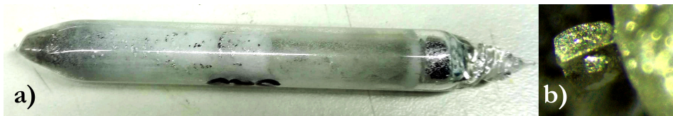
Figure 52: a) Evacuated quartz tube after synthesis filled with crystals, quartz wool, quartz shards, and left over tin (from left to right). b) A cubic crystallite with a small on-growth. This is what the samples are supposed to look like. (Pictures and caption copied verbatim from the Licenciate thesis [3].)
