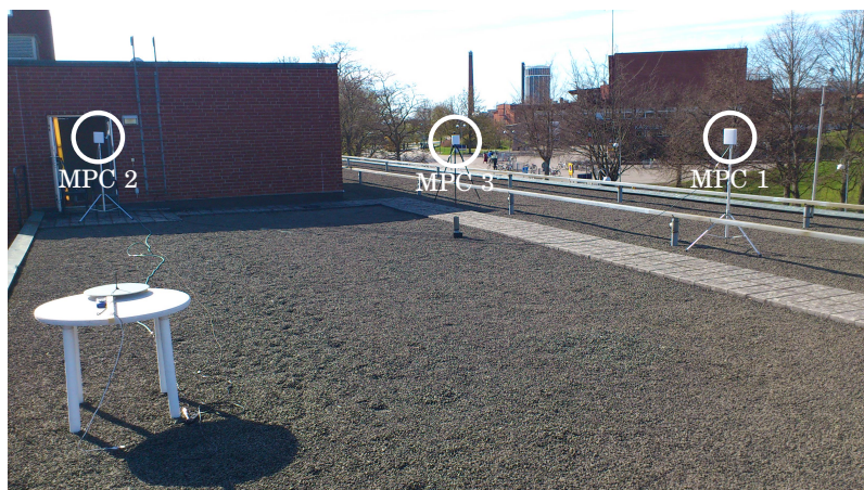
Figure 7.8 The test area with the table holding the IMU and receive antenna closest to the viewer. The three transmitter antennas acting as scattering objects are marked in white.
