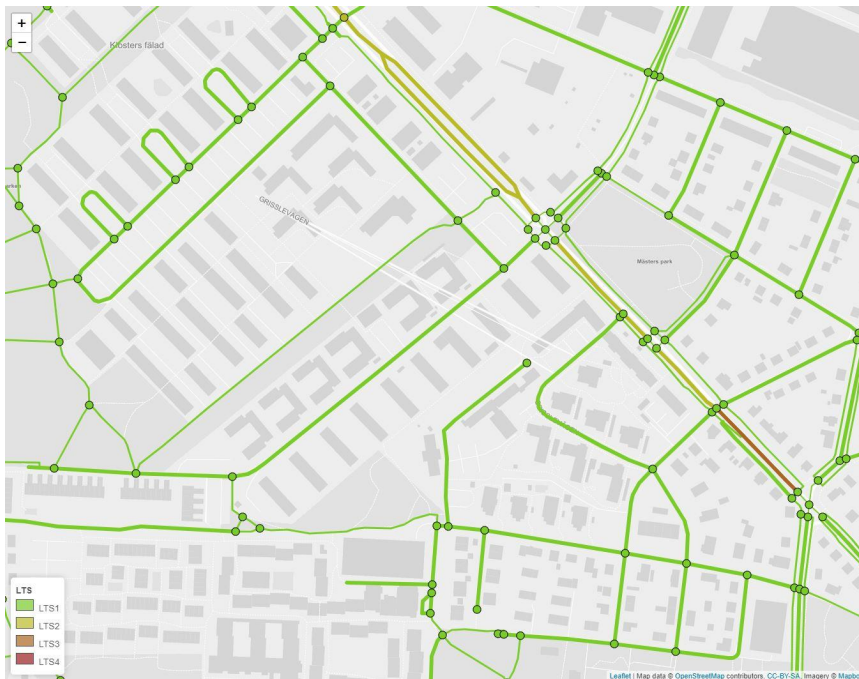
Figure 7. Visualization of LTS values on the map in the study area. The base map is a redistribution of OSM from
