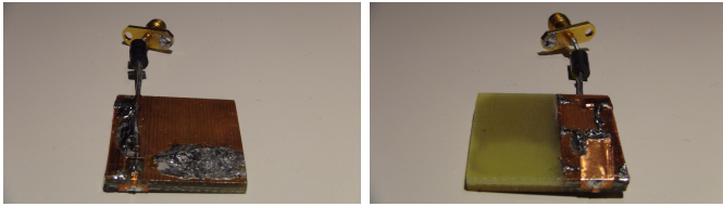
Fig. 5. The GG Antenna, displaying the ground plane on the left and the active element on the right.
