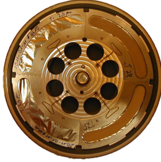
Figure 4.2: Americium target wheel used for the experiment. The target wheel diameter is 10.0 cm. The radial width of the segments is about 8 mm.
