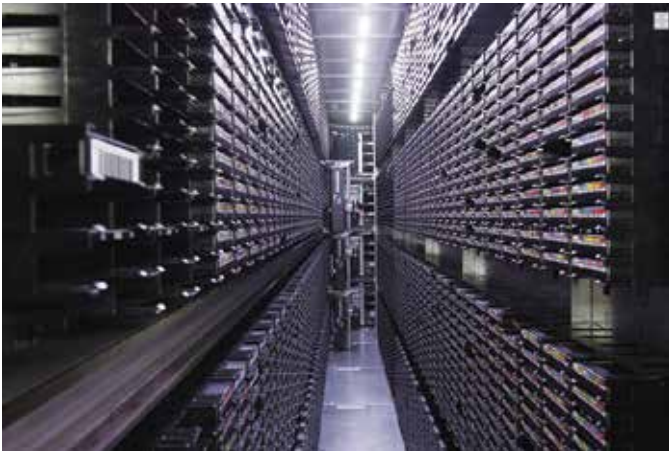
Figure 12. The data storage of climate data at DKRZ where 12 robots services researchers from the whole world, picking up magnetic tapes for reading and distribution of data.
