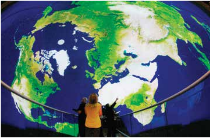
Figure 32. Image from the article “Immersive full-surround multi-user system design” showing how immersants are standing on a gang-plank in an almost total spherical visualization surface in the Allosphere.
