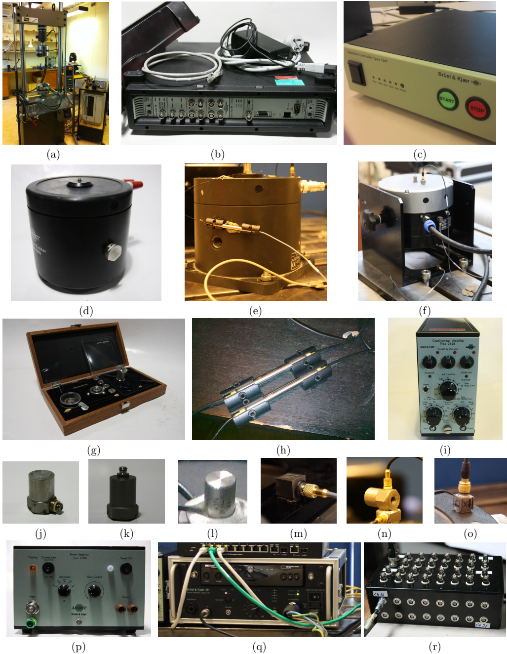
Fig. 4.1: (a) Material testing system MTS 810; (b) Data acquisition system B&K PULSE; (c) Vibration controller B&K 7541; (d) Electrodynamic shaker B&K 4809; (e) Electrodynamic shaker B&K 4808; (f) Electrodynamic shaker B&K 4824; (g) Reference accelerometer B&K 8305; (h) Charge-to-DeltaTron Converter B&K 2647A; (i) Charge amplifier B&K 2626; (j) Accelerometer B&K 4371; (k) Accelerometer B&K 4384V; (l) Accelerometer B&K 4507 001; (m) Accelerometer B&K 4332; (n) Accelerometer B&K 4524B; (o) Accelerometer B&K 4524B; (p) Power Amplifier B&K 2706; (q) Power Amplifier B&K 2734; (r) in-house made connection box for MEMS accelerometers (with built-in power supply).
