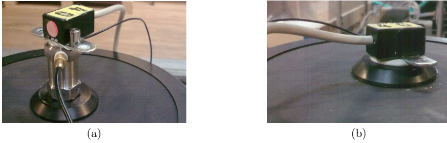
Fig. 7.8: Fixation of MEMS and small B&K 4374 on (a) reference one 8305; (b) directly on shaker.
