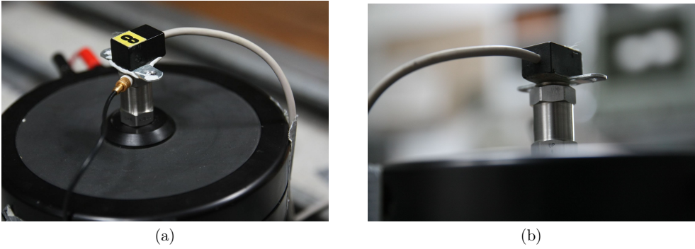
Fig. 7.5: Fixation of accelerometer: (a) using wax; (b) using cyanoacrylate glue.
