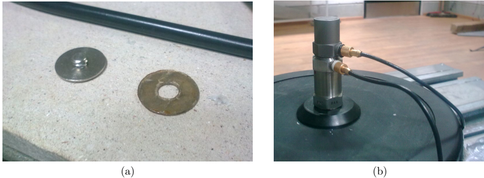
Fig. 7.15: (a) Disk plate and a mica washer; (b) B&K 4371 on the top of B&K 8305.
