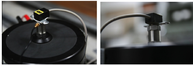
Fig. 4. Details of the fixation of the MEMS to the reference accelerometer and the shaker.
