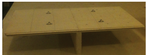
Fig. 2. Dual-plate set-up having flat edges at the junction and no glue applied. The four loops located on the top of the plate were used to hang the structure from the ceiling on rubber springs.
