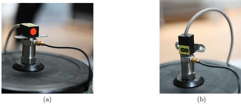
Fig. 7.3: Fixation of the MEMS accelerometer in (a) y - and (b) x -direction.
