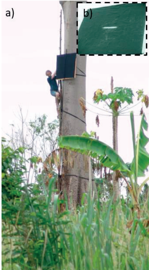
Figure 4.12 Neoprene-covered lidar terminations board mounted in a tree in Ivory Coast. Neoprene is a diffuse scattering target with low reflectance, making it ideal as a termination target in entomological lidar to prevent signal saturation. a) The author is climbing a homebuilt bamboo ladder to mount the neoprene-covered board several meters above ground. Doing so ensures eye safety during measurements. b) The laser beam is centred on the termination target during lidar measurements. The dimensions of the laser spot are used in conjunction with neoprene reflectance to calibrate optical cross sections of insects.
