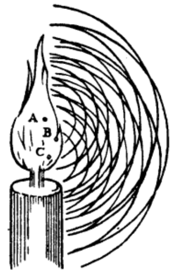
Figure 4.4. Huygens principle states that each point of a light source, like A, B or C, can be assumed as an individual point source that radiate a spherical wave. Figure from the original by Huygens [1690].
