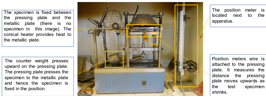
Figure 21: The ISO 5657 ignitability test and its modification for the purpose of measuring material recession rates
