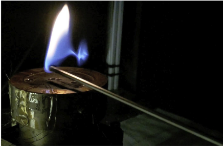
Fig. 2. 50 mm burner and flame igniter.
