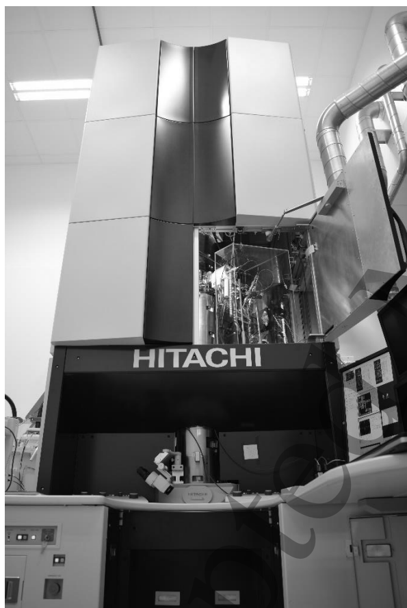
Figure 2 The 300 kV ETEM instrument in Lund. A panel in the microscope enclosure box is open and reveals the sample exchange area. The operator has access to a viewing screen. Pipes into the wall at upper right are for ventilation of the cabinets that house the gas cylinders and the area around the specimen holder at the microscope.
