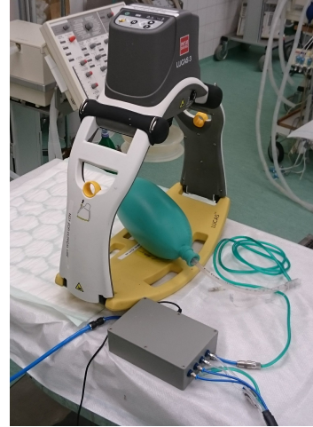
Fig. 5: An mCPR device and the controller (gray box) used to coordinate mCPR and oxygen insufflation during PIIO, with a balloon representing the lungs.
