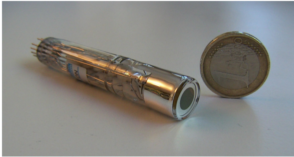
Figure 4.2.: R760 Hamamatsu PMT with specially reduced sensitive window size used in the LUCID detector.
