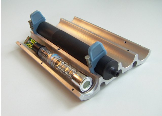
Figure 4.15.: Metal support for the PMT tubes that is used in the LUCID detector.
