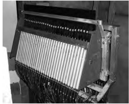
Figure 3: The focal plane hodoscope shown in position next to the main tagger.
