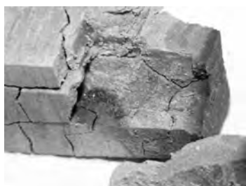
Figure 1. Example of a clay ring exhibiting signs of reduction. The inner part of Calcigel block #5 showing a radial change in colour (the dark part to the right was in direct contact with the iron heater). The cracking of the clay is due to dehydration in the dry glove-box.
