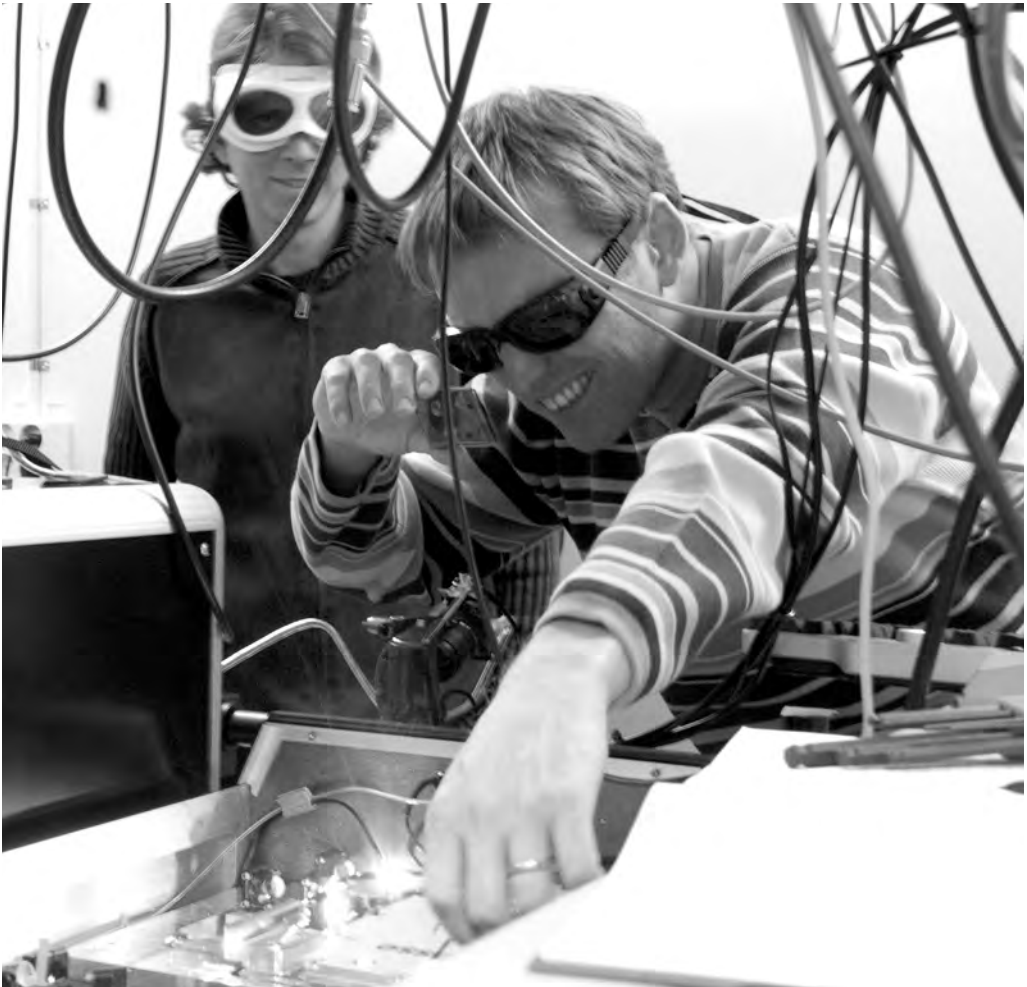
Filip Lindau assisted by Christian Erny aligning the Ti:sapphire laser oscillator in the laser hutch. The oscillator is part of the testFEL laser system, seeding amplifiers that generate UV laser pulses both for the RF photocathode gun and the FEL seed laser, May 2009. Photo: Nino Čutić
