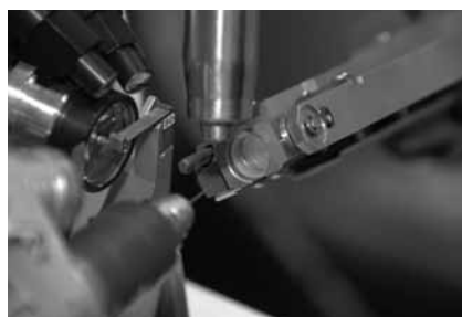
Figure 2: Sample holder on the mini-kappa (lower left) with sample changer tool (upper right), cryo nozzle (top), on-line viewing and sample illumination (upper left) with the triple aperture in the centre of the lens.
