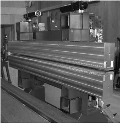
Figure 1: The I311 undulator with the upgraded magnetic structure in July 2010.
