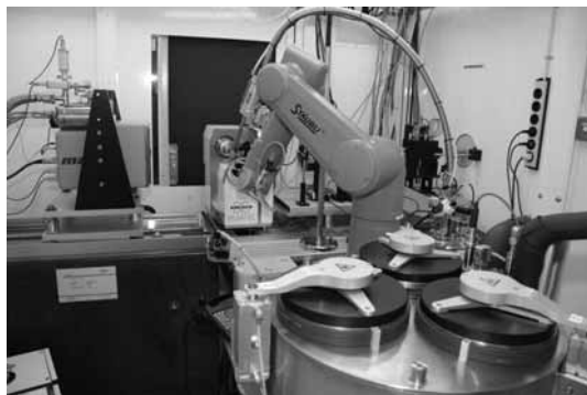
Figure 3: The new I911-3 experiment set-up with the robot of the sample changer in the centre. The area detector can be seen to the left on its granite support.
