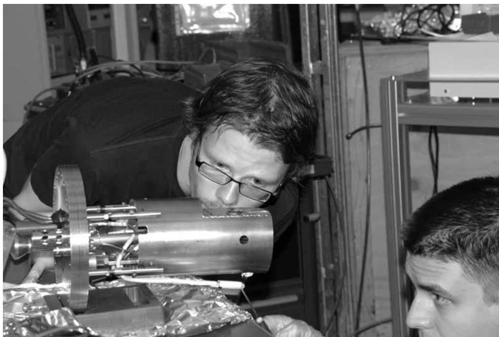
Mikko-Heikki Mikkela, University of Oulu, and Samuli Urpelainen, fine tuning the evaporation oven of the exchange metal cluster source at beamline I411, 11 October 2010. Photo: Annika Nyberg
