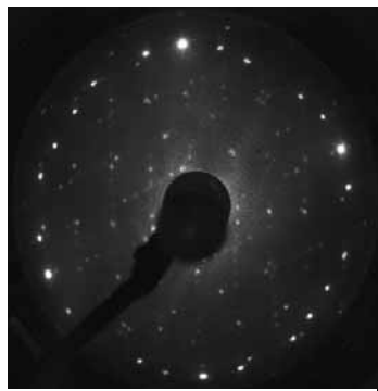
Figure 2. A LEED pattern from the C/Fe(110) sample. E_p=102 eV.
