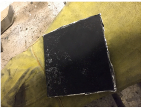
Polymer Specimen and Aluminum foil backing
