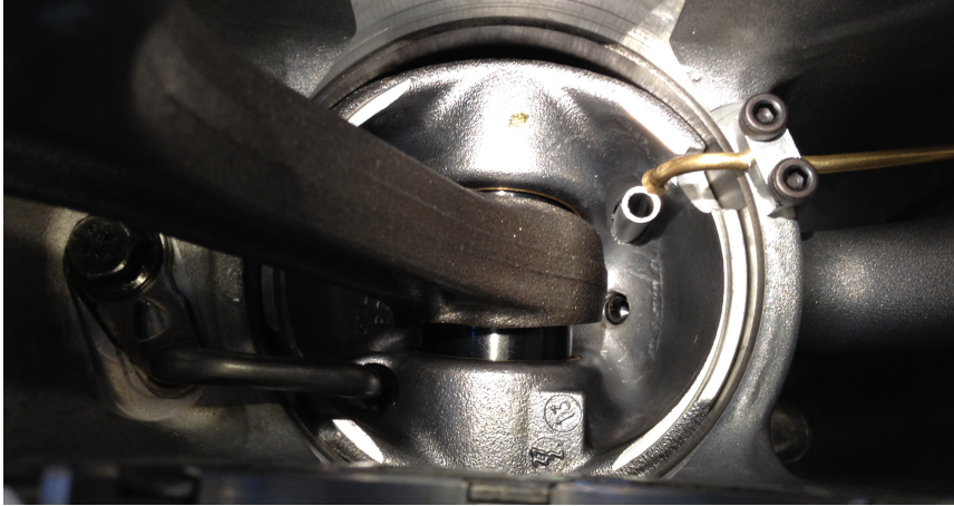
Figure 4.3: Position of thermocouple measuring piston oil return flow temperature.
