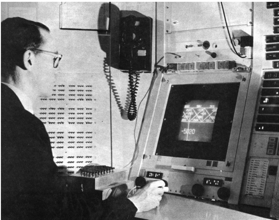
Figure 4.3: Sketchpad - the first CAD tool
