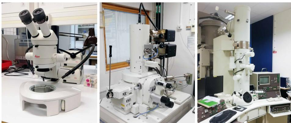
**Figure 1.2:** Three different microscopes that all have been used during the thesis. From left to right: A visual light microscope (VLM, Leica), a scanning electron microscope (SEM, Jeol JSM-6700F), a transmission electron microscope (TEM, JEM-3000F).
