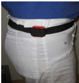
Fig. 10. An accelerometer on a belt on the right hip.
