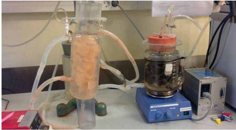
Figure 5 The lab-scale setup used in Paper III , with an aerated reactor containing Z200 (left) and an anaerobic, mechanically stirred reactor containing K5 (right).
