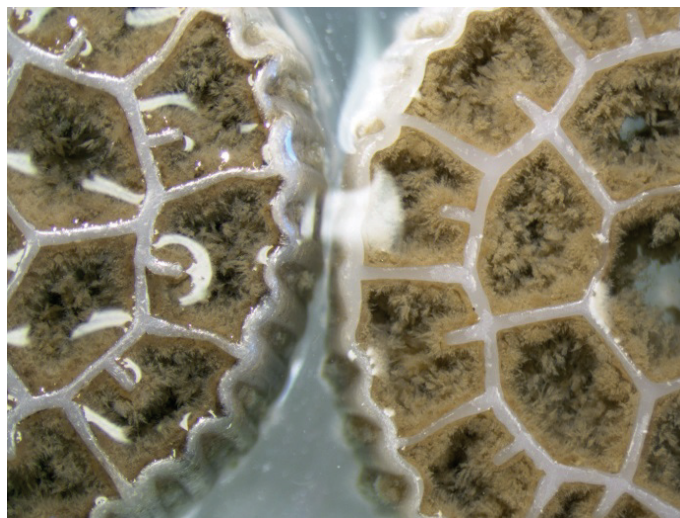
Figure 19 K3 carriers from the municipal treatment plant, as taken from the N-stage on the 11 th of April, 2014.
