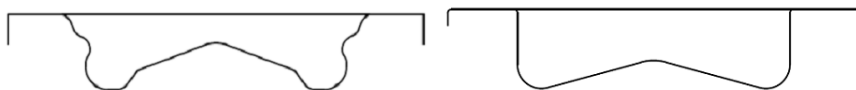
Figure 4.2: The two engine piston used in the experiments (the original one to the left and the modified one to the right).
