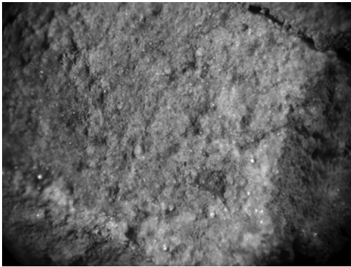
Fig. 15. Microscope photo of inside of crucible with small round drops most likely of gold (a) x15 and polished section of the same crucible showing an outer repair layer to the left (b) x4. Square 1b.
