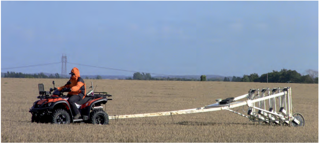
Fig. 2. Magnetic survey at Uppåkra in August 2010 with motorized 5-channel Foerster gradiometer array mounted on a non-magnetic cart. The RTK-GPS antenna for data positioning is visible on the cart. Data logging and navigation is implemented using LBI ArchPro LoggerVIS1.0 software on a rugged laptop in front of the operator.
