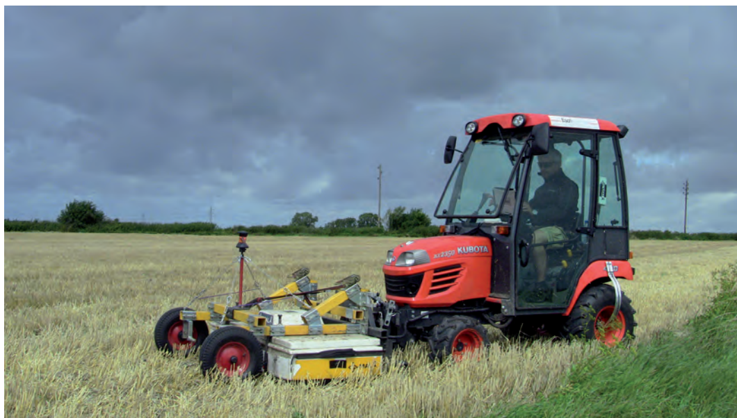
Fig. 3. Motorized GPR measurements with the 16 channel 400 MHz MALÅ Imaging Radar Array (MIRA) with 8×8cm spatial resolution tracked by a robotic totalstation.
