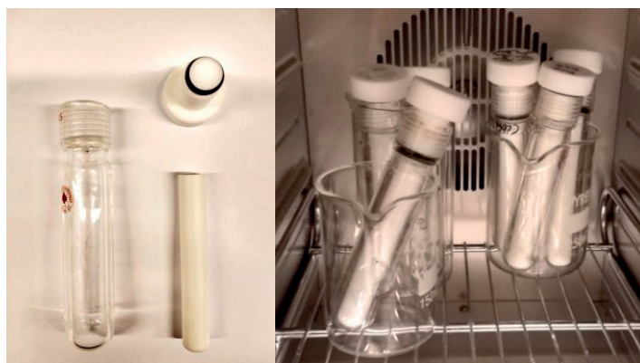
Figure 14. Sample holders used to store samples in alkaline media for alkaline stability assessment at >80 °C. Left: pressure safe glass container with screw cap and a special made Teflon insert. Right: Assembled holders in an oven.
