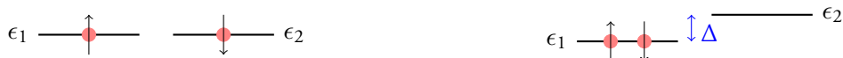
Figure 6.3: Detuning between the single electron energy levels in the quantum dots. The two-electron ground state changes when detuning the one electron levels. When the detuning becomes strong enough to overcome the Coulomb repulsion, the S(2,0) becomes the ground state.
