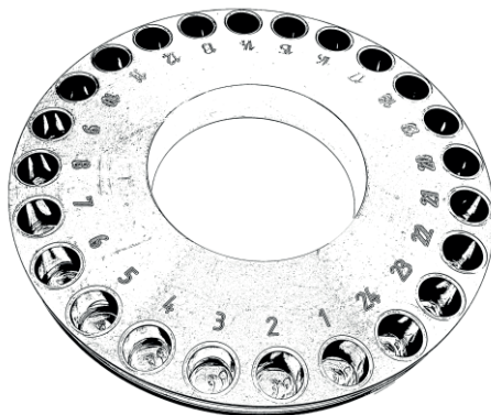
Figure 10. NACIVT chamber well plate for simultaneous aerosol exposure to 24 cell cultures at the ALI.
