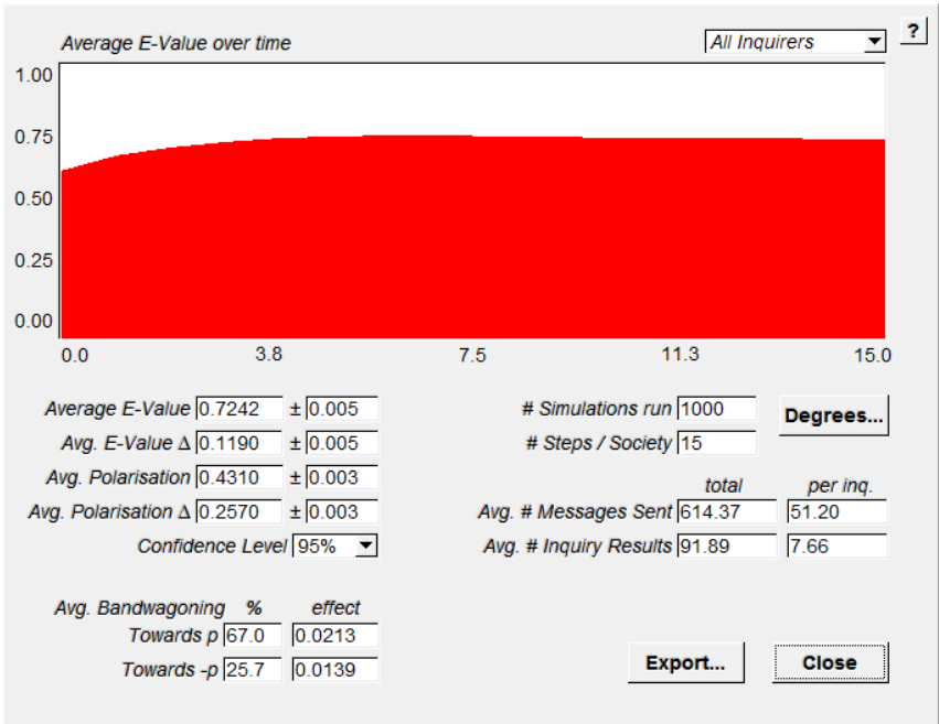
Figure 6: Typical result of simulation in batch mode with increase in epistemic value as well as polarization. E-value has increased by 0.1190 and polarization has increased by 0.2570.
