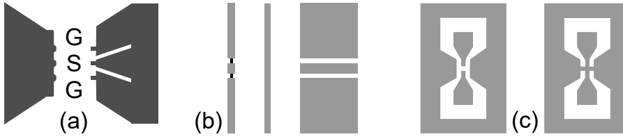
Figure A.2: (a) Schematics of two different kinds of RF probes. (b) Calibration structures for LRRM calibration: 50\ \Omega , short, 'thru'. (c) De-embedding pads, 'open' (left) and 'short' (right).
