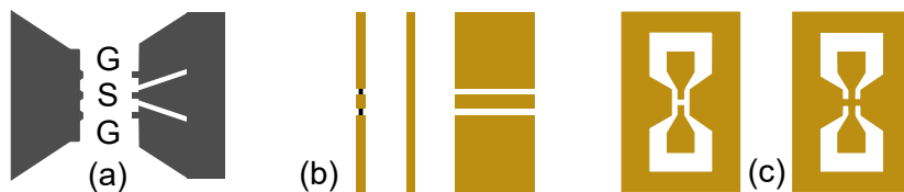
Figure 1: Schematics of (a) two different RF probes, (b) the calibration structures used for an LRRM calibration (from left to right: load, short, through), and (c) open (left) and short (right) de-embedding structures to remove the effect of the transistor contact pads.
